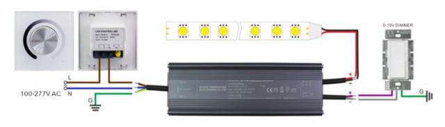
Input Wire: 18AWG Black and White to be connected to AC Line (L) and Neutral (N), Green Wire connect to Ground Output Wire: 16AWG Red to LED Positive Side (+), Black to LED Negative side (-). Purple (+) and Gray (-) Wires to 0-10V Dimming
