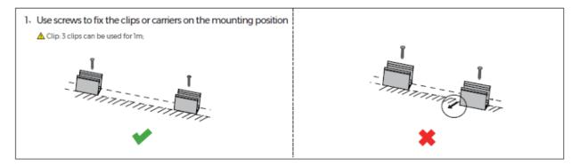
Installation into linear channels or substrates - It is recommended to use caution when inserting the strip into channels and various substrates. LED is not meant to have sharp bends, so make sure to use extreme caution when inserting or removing the strip from a channel.
