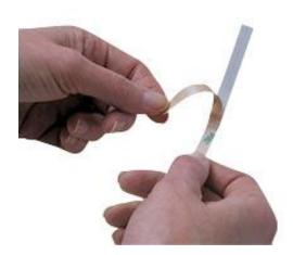
Make sure the LED Strip runs linearly along on the same plane to avoid awkward bending of the strip. This LED Strip is meant to move up and down, like a roller coaster. Not side to side.
