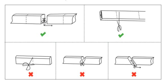
Once the LED is cut, use flush cutters or razor blade to expose the backside of the LED strip. The backside is the same side as the cut marks on the side of the jacket.
