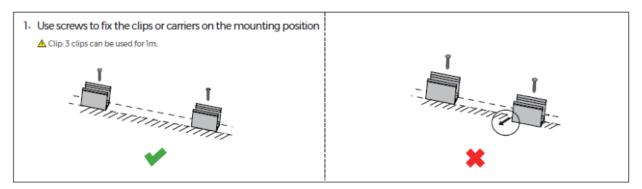
Installation into linear channels or substrates - It is recommended to use caution when inserting the strip into channels and various substrates. LED is not meant to have sharp bends, so make sure to use extreme caution when inserting or removing the strip from a channel. When installing long lengths, 2-person installation is recommended to avoid damaging the LED Strip.
