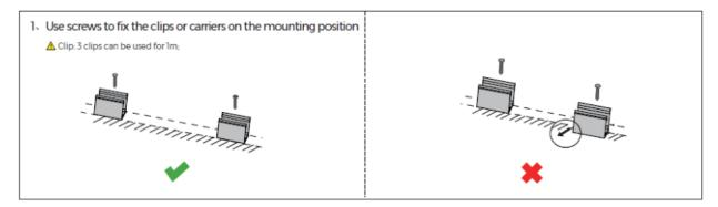
Installation into linear channels or substrates - It is recommended to use caution when inserting the strip into channels and various substrates. LED is not meant to have sharp bends, so make sure to use extreme caution when inserting or removing the strip from a channel. When installing long lengths, 2-person installation is recommended to avoid damaging the LED Strip.
